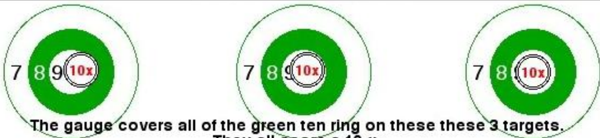
If you see any green of the 10-ring peeking out from under the edge of the gauge, it is not a 10x.
